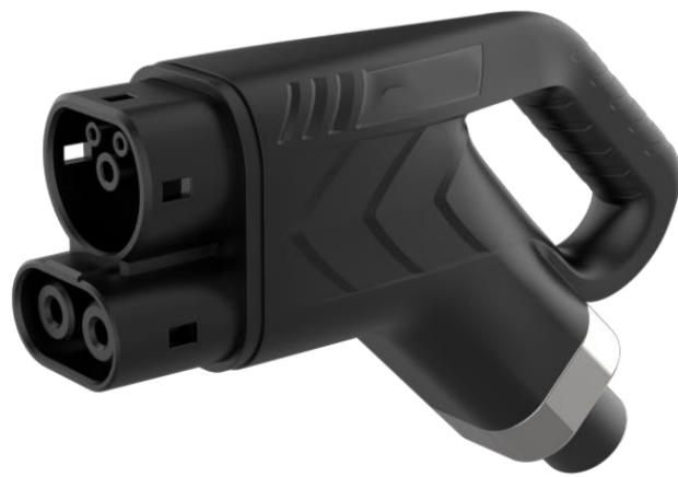
The CCS2 Plug with replaceable DC terminals and mounting surface frame. It is installed on the electric vehicle charging pile, charging mode 4, and is used to quickly charge electric vehicles with direct current (DC) through the CCS2 type vehicle socket. The product meets IEC62196.3-2022 and RoHS2.0 requirements.
